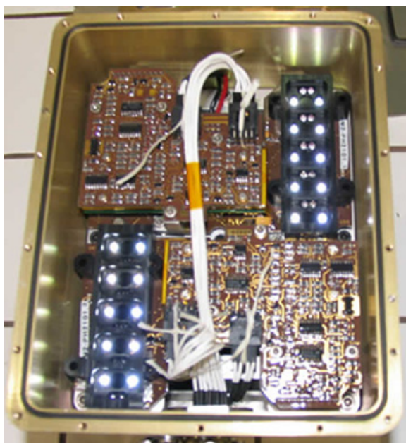
Figure 6. Picture of the instrument at the end of fabrication, showing the electronic control and measurement boards and the optical modules with the LEDs on. The biological container arrays to be placed over the optical modules are still unmounted.
